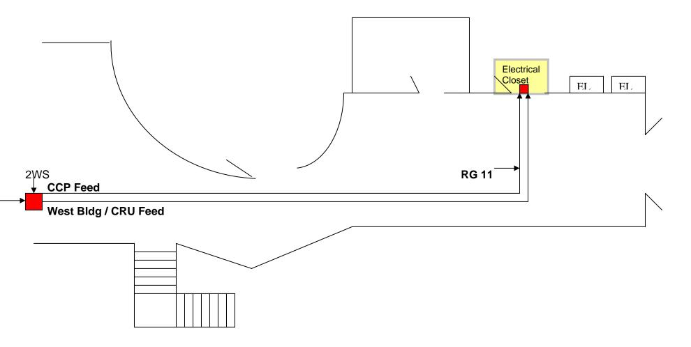
Legend: 2WS= Two way signal splitter @ 3.5db signal drop EL = Elevator
