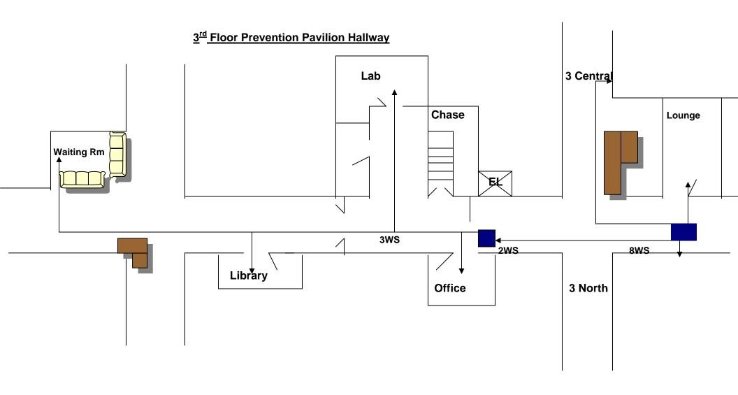
**Legend: 2WS = Two way signal splitter** 3WS = Three way signal splitter 8WS = Eight way signal splitter
